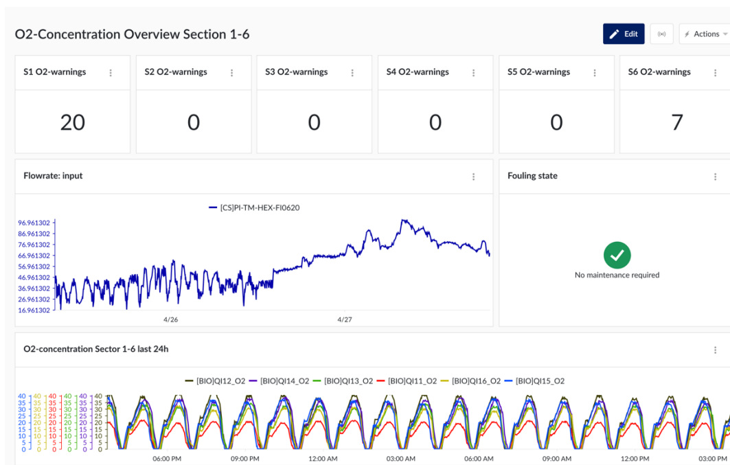
Figure 1. Maintenance Dashboard to monitor the fouling state of aeration elements.
