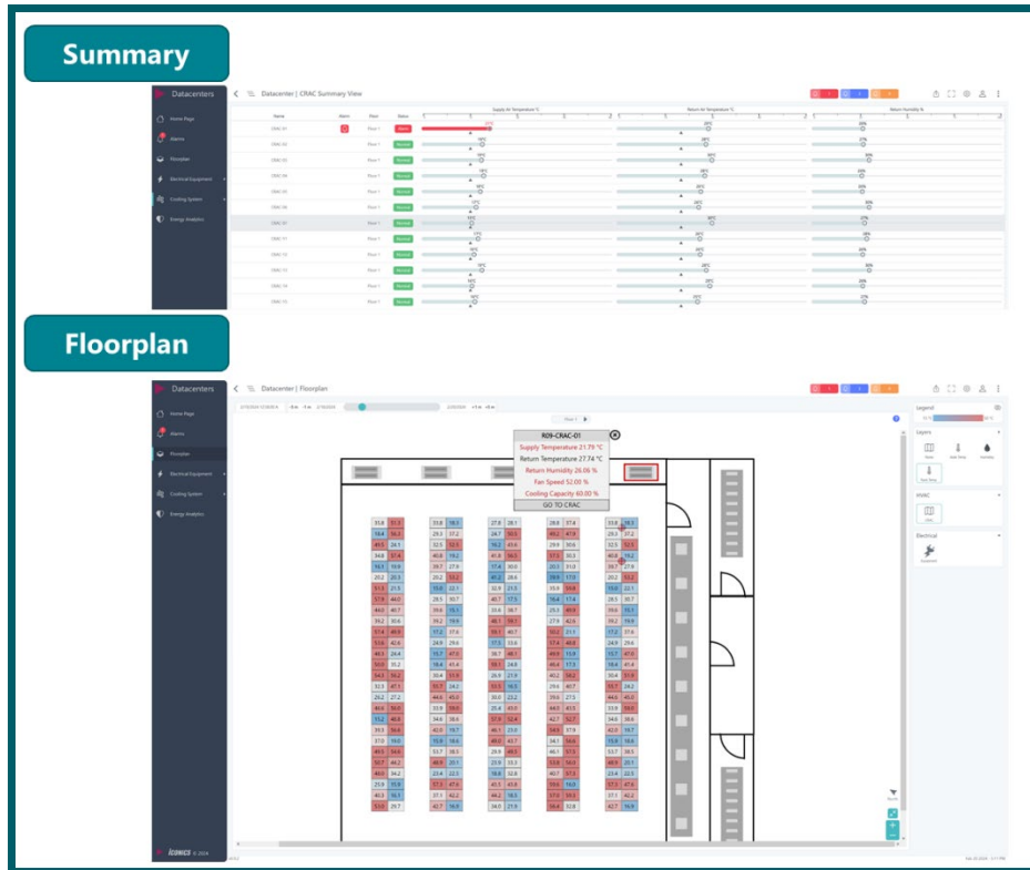
Figure 3. A “single pane of glass” providing a holistic view of a data center’s operations.
